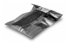
This static shield bag offers total ESD protection, whether you're transporting ESD-susceptible products across the room or across the country. The outer layer of the bag consists of an abrasion-resistant polyester, while the antistatic polyethylene inner layer retards triboelectric static charging from inside the bag.
